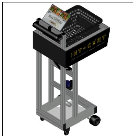
**Fig. 1.** 3D model of int-cart
