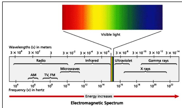
Fig. 4. Electromagnetic spectrum [20]
