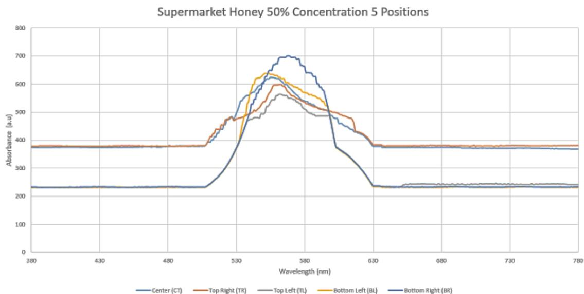
**Fig. 6.** Graph of absorbance vs. wavelength of supermarket honey with 50% concentration measured at 5 different positions
