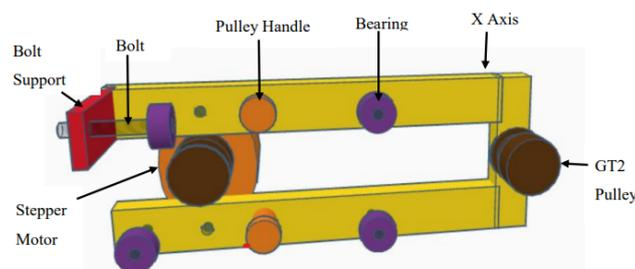
**Fig. 2.** X axis section of the proposed spectroscopy
