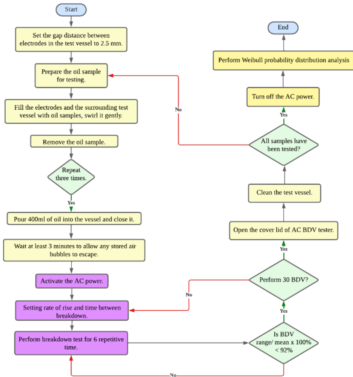
Fig. 1. Flowchart of the AC breakdown voltage experiment process
