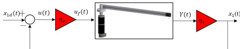
Fig. 1. Multiplicative fault as the basic fault models for SLFM system
