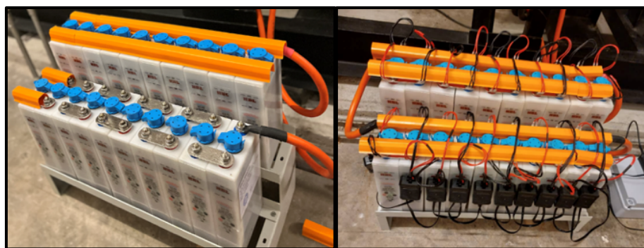
Fig. 2. Battery packs without (left) and with (right) the installed BMS
