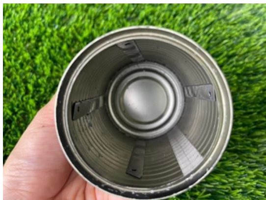
Fig. 5. Bar fixed were added into the mill jar
