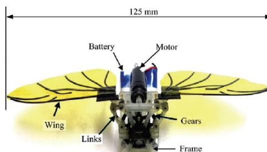
**Fig. 9.** Modified flapper model [63]
