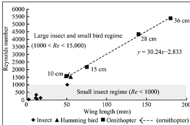
Fig. 5. Reynolds number versus wing length [45]
