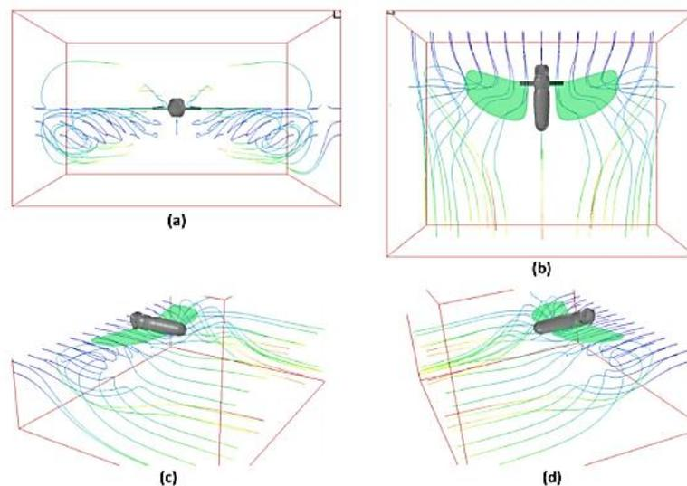
**Fig. 10.** Flow patterns under MAV during half stroke at different views (a) Front (b) Top (c) Left 3D (d) Right 3D [65]
