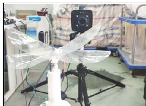
**Fig. 7.** Phase angle identification setup using ellipse wing profile with 260 mm of wingspan [2]
