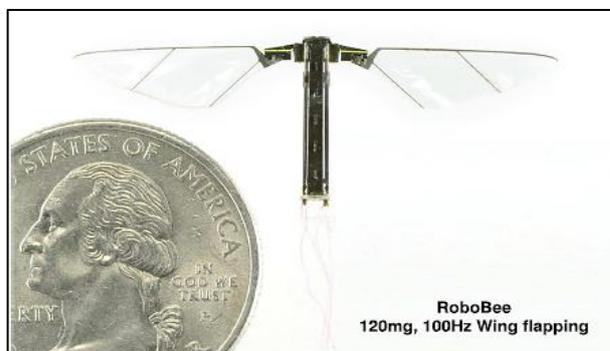
**Fig. 6.** RoboBee is a biologically inspired bee-sized micro air vehicle [57]
