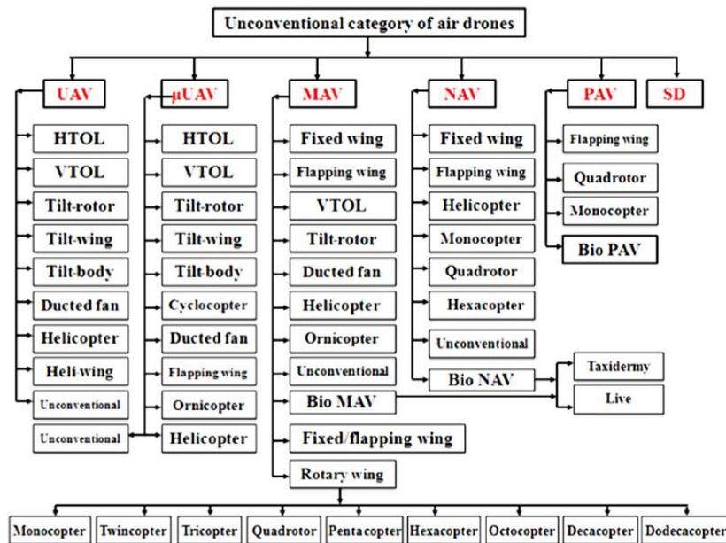
Fig. 1. Different types of air drones [3]
