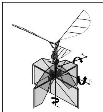
**Fig. 2.** A novel flapping wing rotary MAVs invented by Dong *et al.*, [16]
