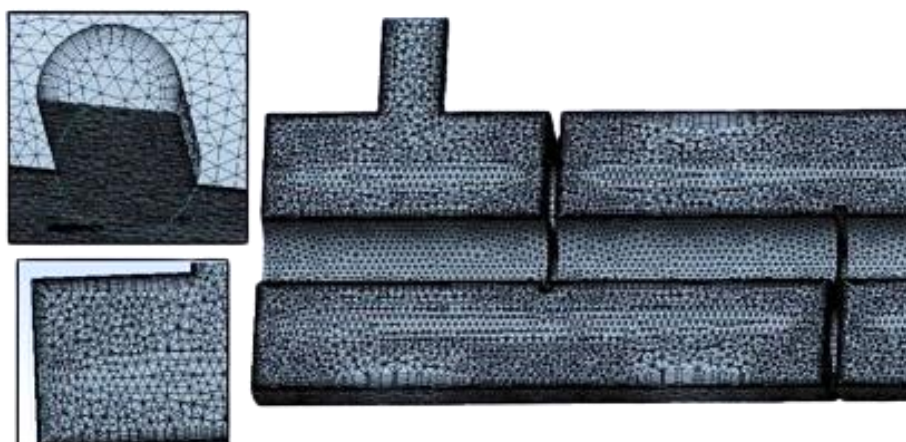
Fig. 7. Initial inflation layers
