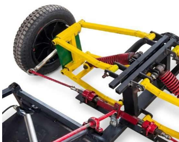
Fig. 7. Fabricated double-wishbone based on the design and analysis using hollow carbon steel
