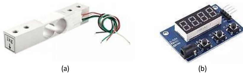
Fig. 1. Experimental instrumentation (a) Shear beam load cell sensor (b) V774 digital decoder module
