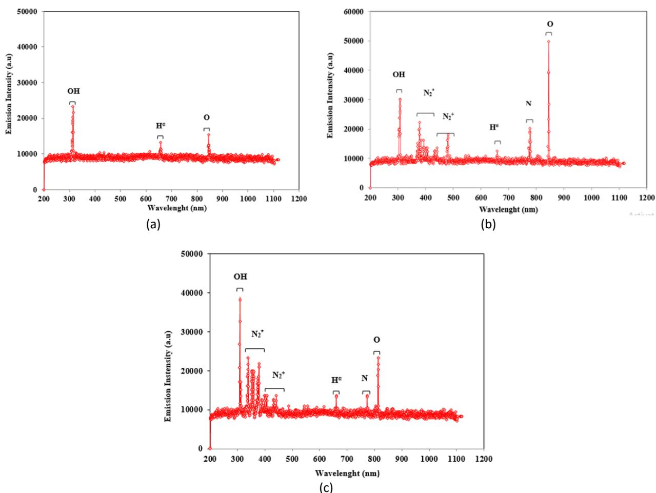
**Fig. 3.** Emission intensity of radical production (a) without air injection (b) with air injection (c) with air injection and addition of  $\text{Fe}^{2+}$  ions
