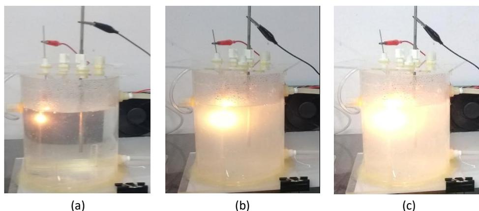
**Fig 2.** Plasma electrolysis process (a) without air injection (b) with air injection (c) with air injection and addition of  $Fe^{2+}$  ions
