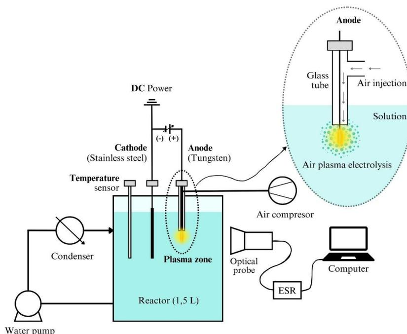
Fig. 1. Plasma electrolysis reactor setup
