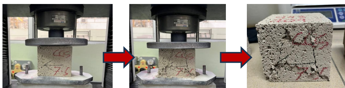
Fig. 3. Compressive strength test
