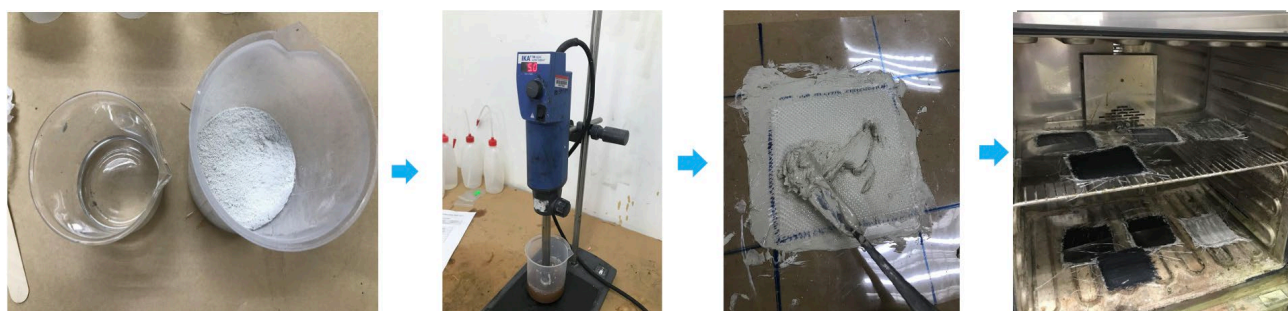
Fig. 1. Glass fiber reinforced geopolymer composites (GFRGCs) fabrication process
