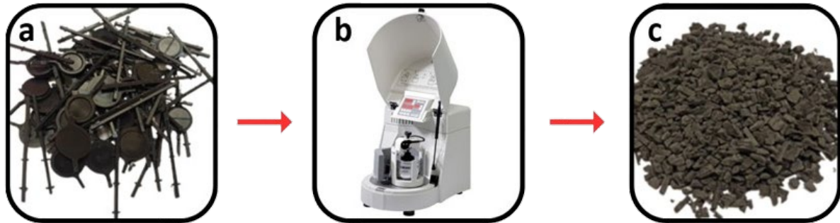
Fig. 1. Material preparation (a) Resin waste (RW) from IC packages electronic industry; (b) Grinder Machine Fritsch's Planetary Mono Mill Pulverisette 6 Classic Line (c) Grinded resin waste
