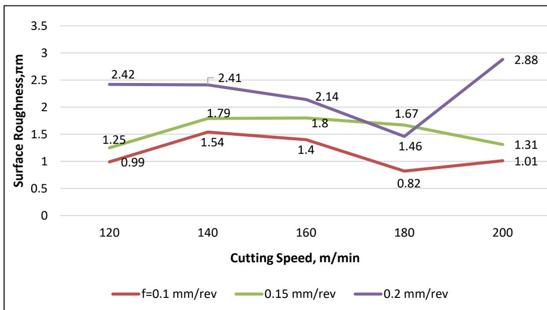
**Fig. 9.** Graphic of cutting speed vs surface roughness of the workpiece in different cutting feed
