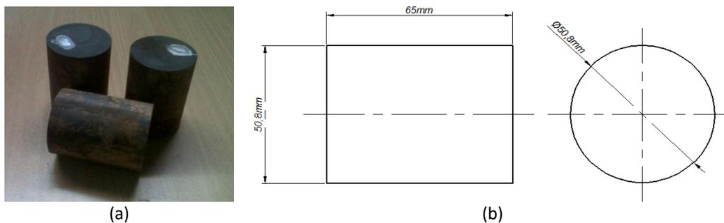
**Fig. 3.** (a) AISI D3 Steel workpiece (b) Workpiece specification
