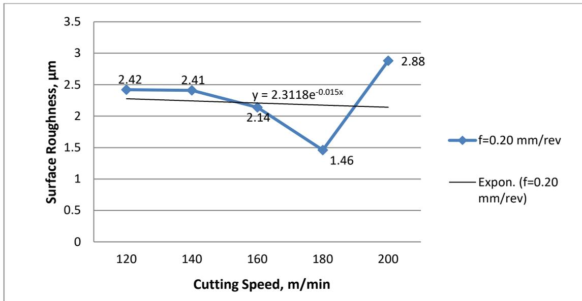
**Fig. 8.** Graphic of cutting speed vs surface roughness of the workpiece where cutting feed, f is 0.20 mm/rev
