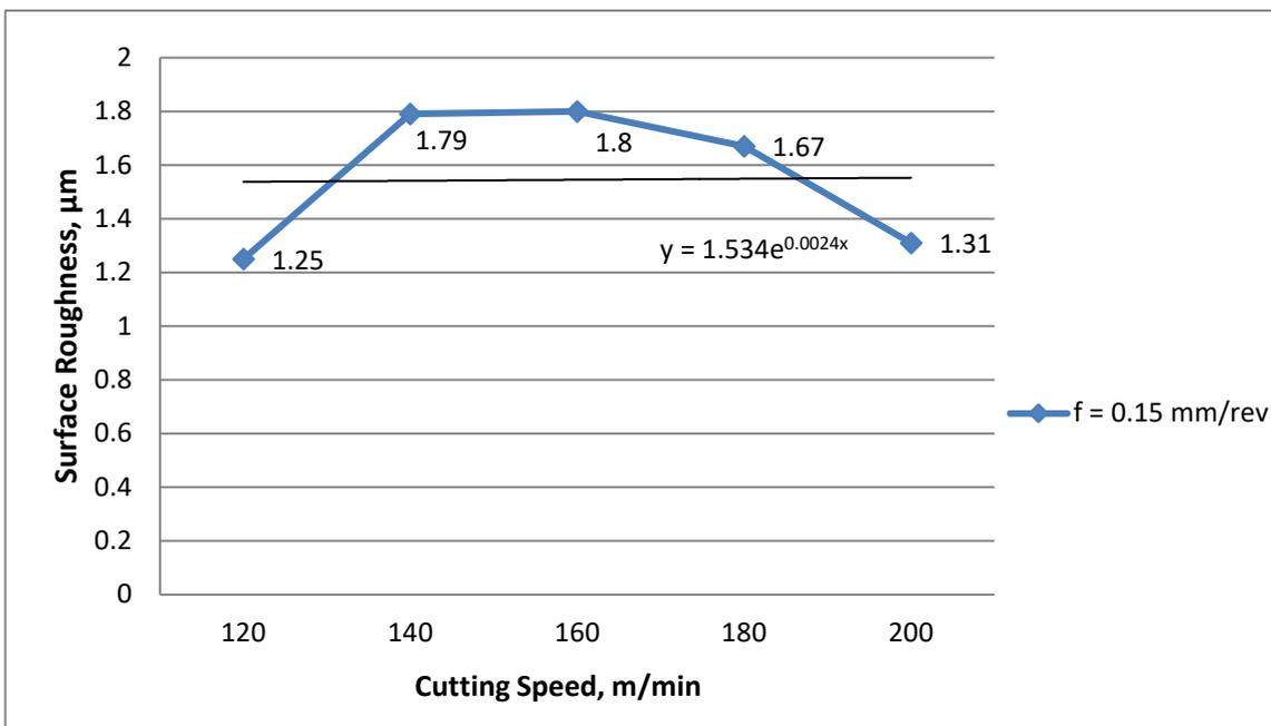
**Fig. 7.** Graphic of cutting speed vs surface roughness of the workpiece where cutting feed,  $f$  is 0.15 mm/rev
