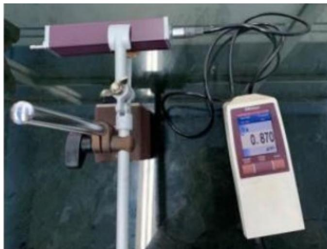
**Fig. 2.** Surface tester Mitutoyo
