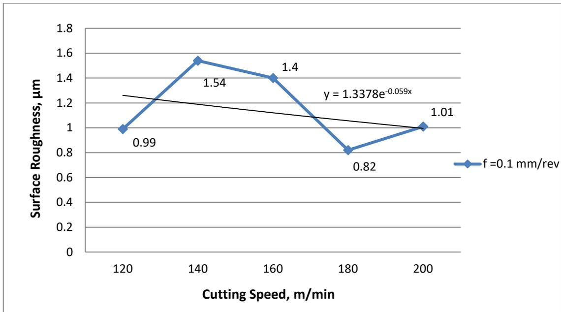
**Fig. 6.** Graphic of cutting speed vs surface roughness of the workpiece where cutting feed,  $f$  is 0.1 mm/rev
