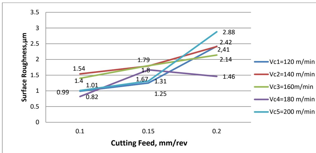
Fig. 10. Graphic of cutting feed towards surface roughness in different cutting speed
