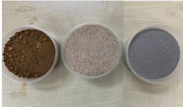
**Fig. 2.** Image capture of actual samples used soil, sand (medium-sized grain), and cement (powder form)
