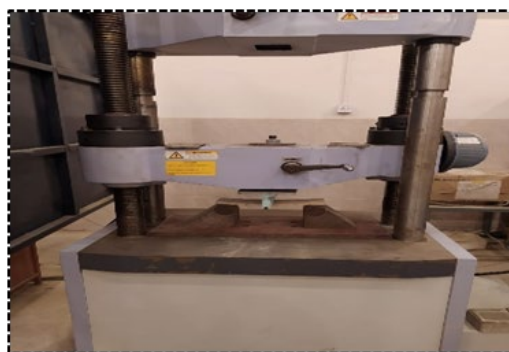
Fig. 5. Flexural strength Testing setup
