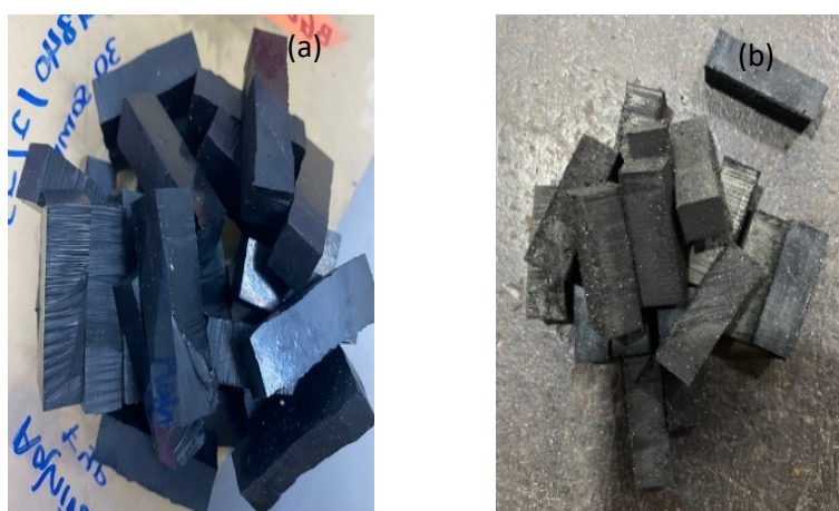
Fig. 1. Samples were cut using a special cutter for (a) DPNR-25 and (b) DPNR-50
