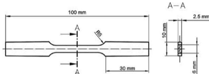
Fig. 2. Dimension of the dog bone according to the ASTM E8
