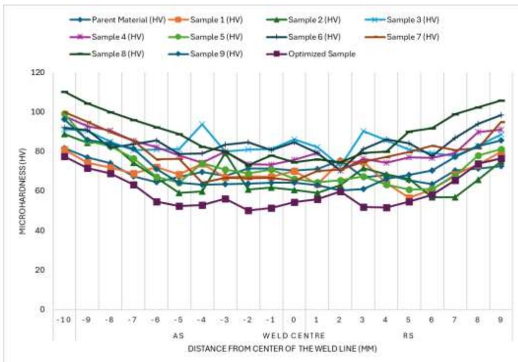
**Fig. 4.** Graph of microhardness (HV) vs distance from centre of the weld line
