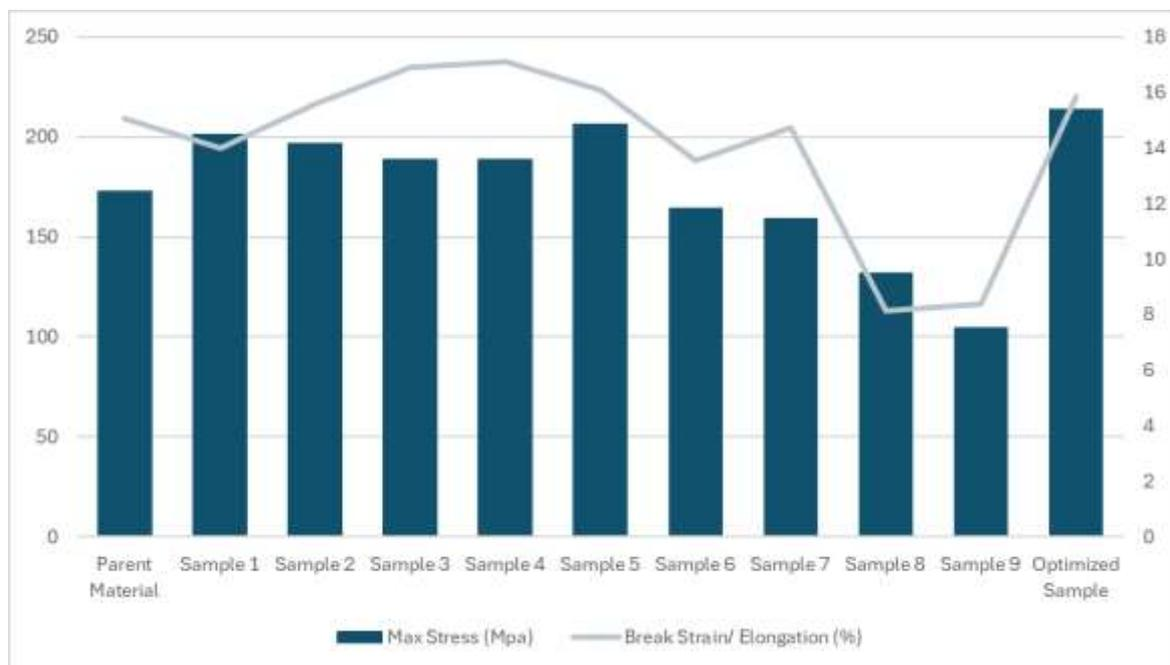
**Fig. 3.** Graph UTS (MPa) and and Break Strain/Elongation (%)
