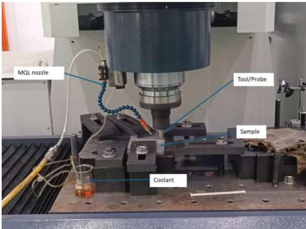
**Fig. 1.** Cooling system setup
