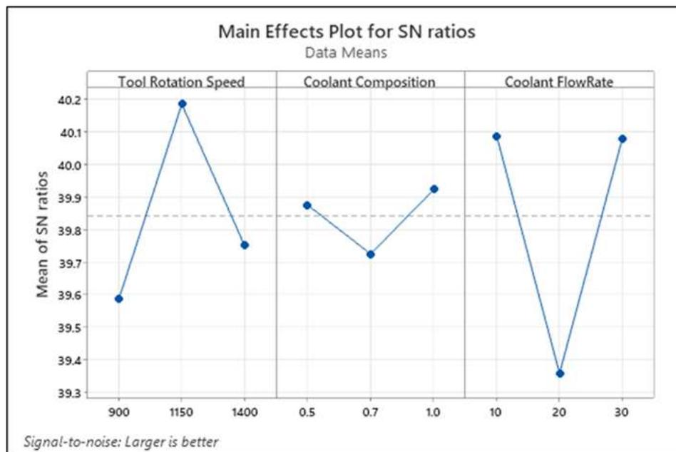
Fig. 5. 3 Graph of main effects plot for SN ratios by Minitab software
