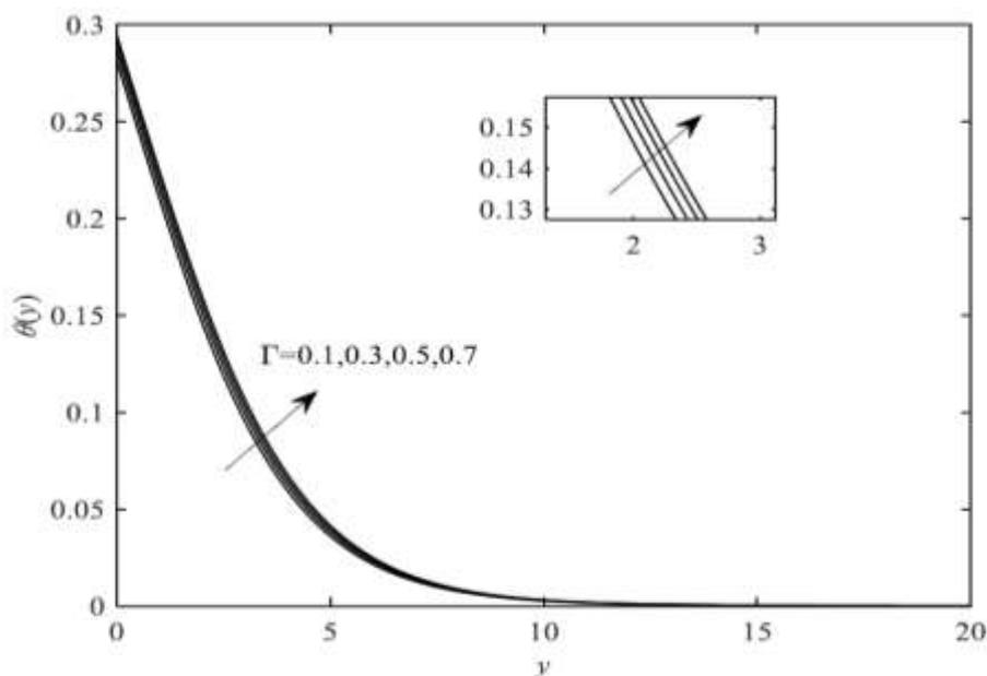
**Fig. 6.** Temperature profile,  $\theta(y)$  for a variety of  $\Gamma$  with  $k_1 = 1$  and  $Bi = 0.1$
