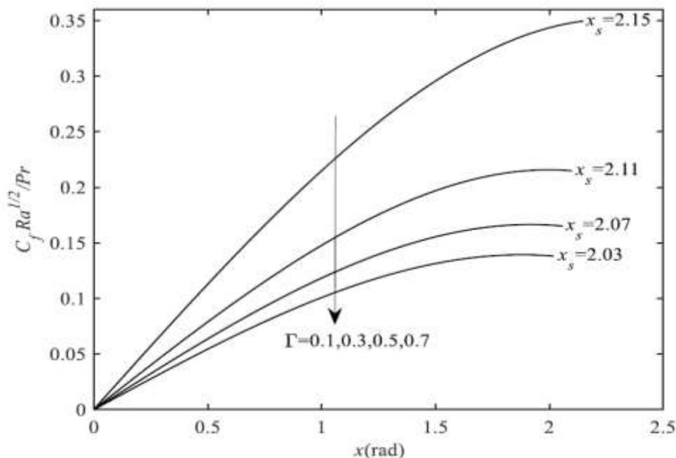
**Fig. 9.** Skin friction coefficient,  $C_f Ra^{1/2} / Pr$  for a variety of  $\Gamma$  with  $k_1 = 1$  and  $Bi = 0.05$
