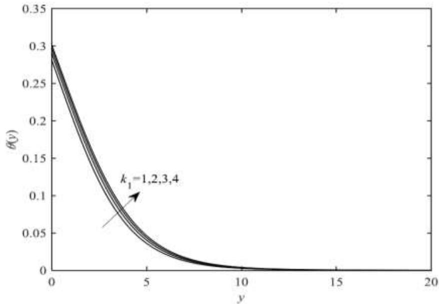
Fig. 4. Temperature profile,  $\theta(y)$  for a variety of  $k_1$  with  $\Gamma = 0.1$  and  $Bi = 0.1$
