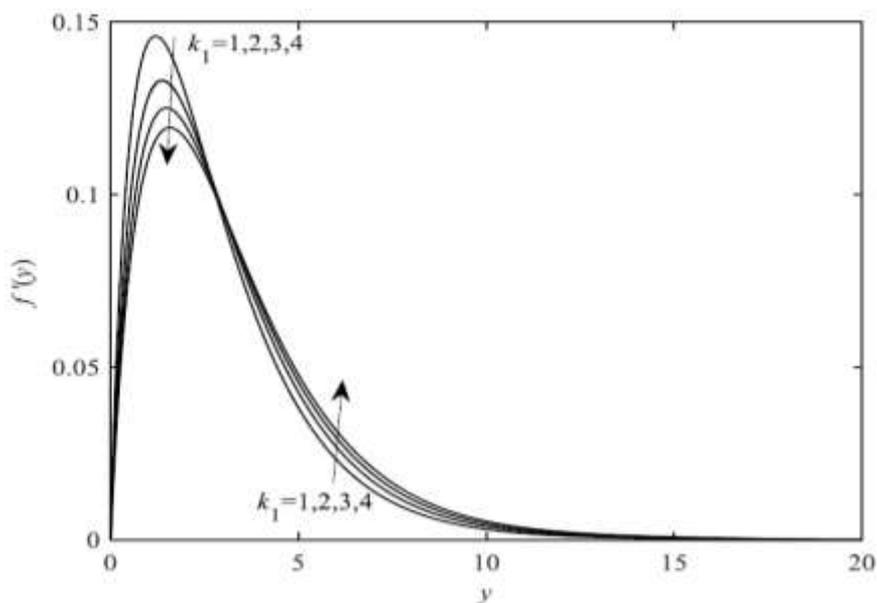
**Fig. 3.** Velocity profile,  $f'(y)$  for a variety of  $k_1$  with  $\Gamma = 0.1$  and  $Bi = 0.1$
