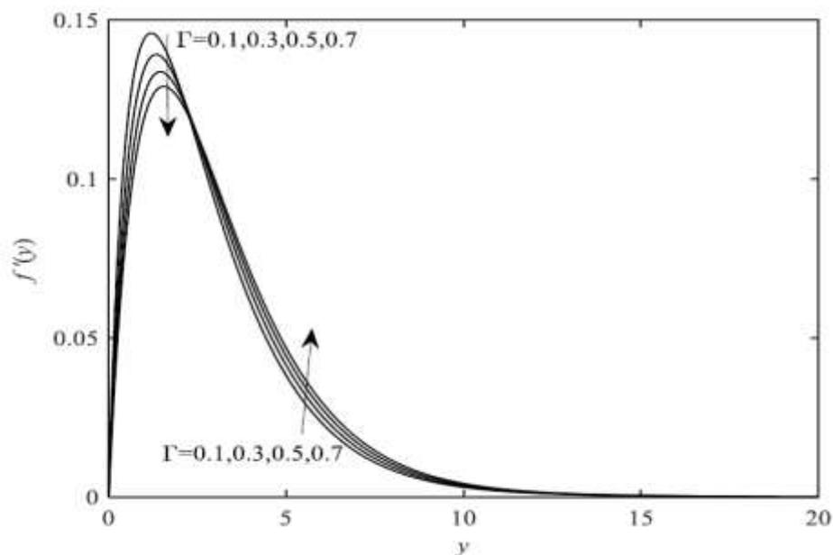
Fig. 5. Velocity profile,  $f'(y)$  for a variety of  $\Gamma$  with  $k_1 = 1$  and  $Bi = 0.1$
