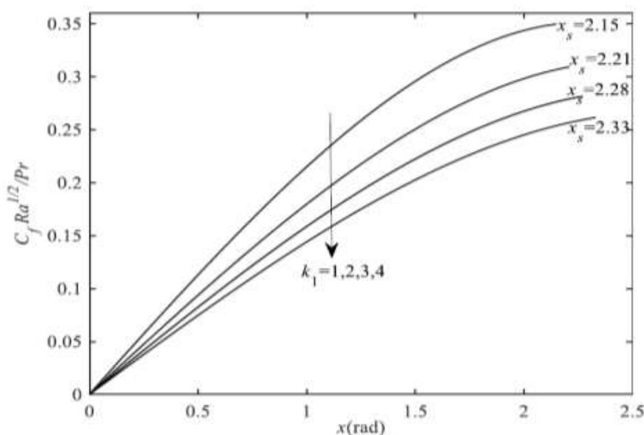
**Fig. 7.** Skin friction coefficient,  $C_f Ra^{1/2} / Pr$  for a variety of  $k_1$  with  $\Gamma = 0.1$  and  $Bi = 0.05$
