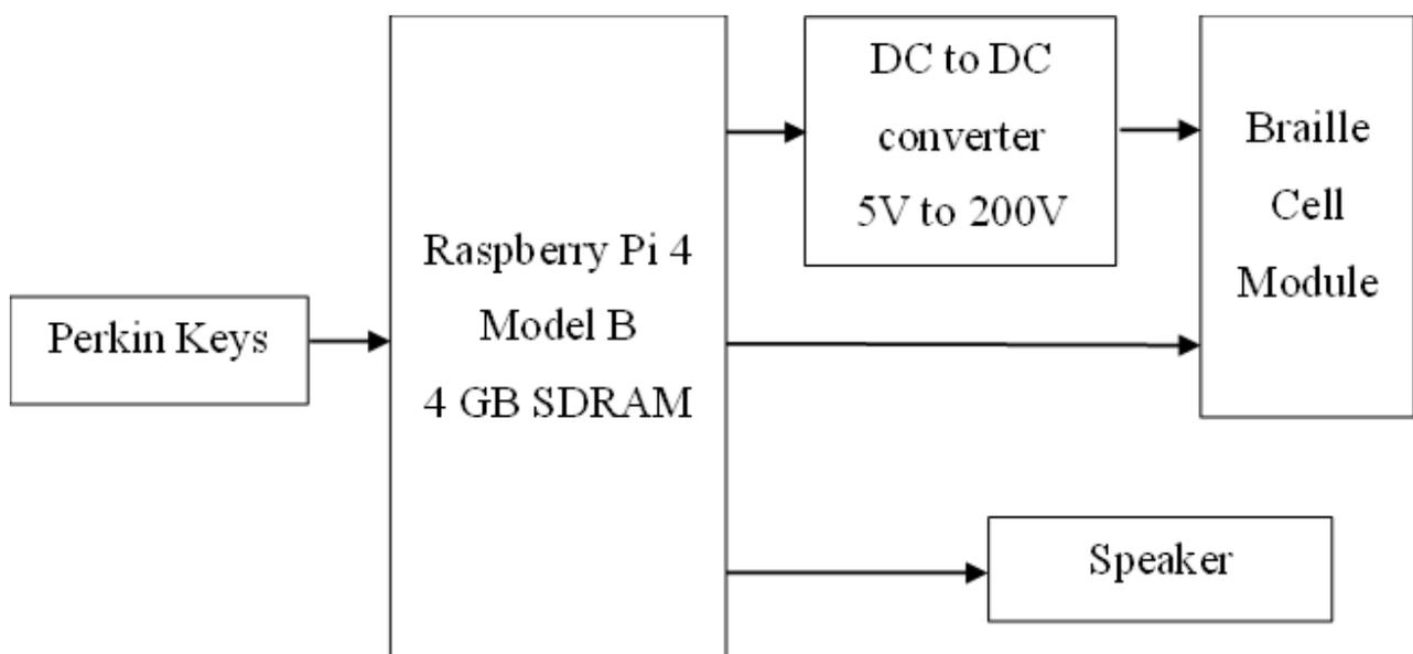
Fig. 1. The block diagram of the braille notetaker
