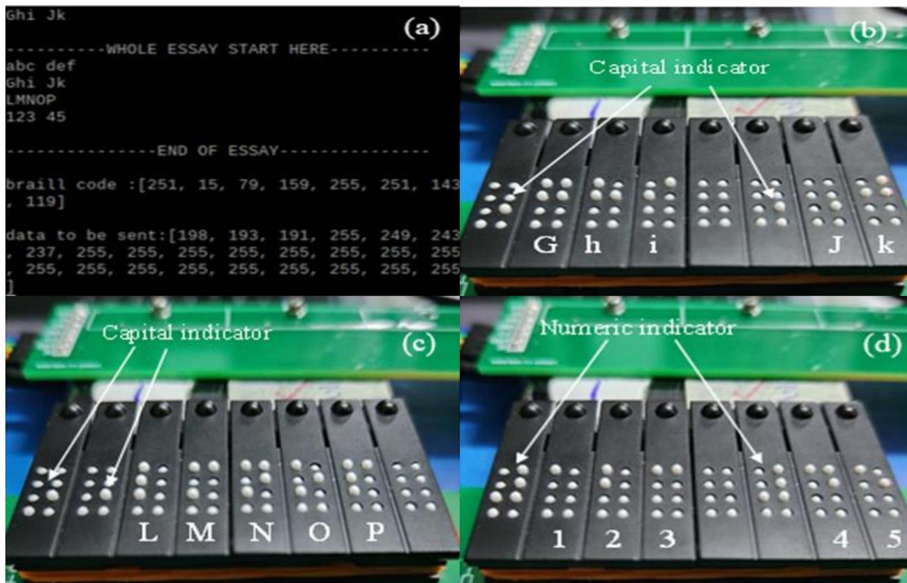
**Fig. 3.** (a) The terminal of Raspberry Pi 4 (b) The second line of the essay (c) The third line of the essay (d) The fourth line of the essay
