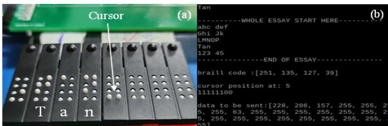
**Fig. 4.** (a) The cursor is shown on the 5<sup>th</sup> braille cell (b) The new word “Tan” is shown on the terminal of Raspberry Pi 4
