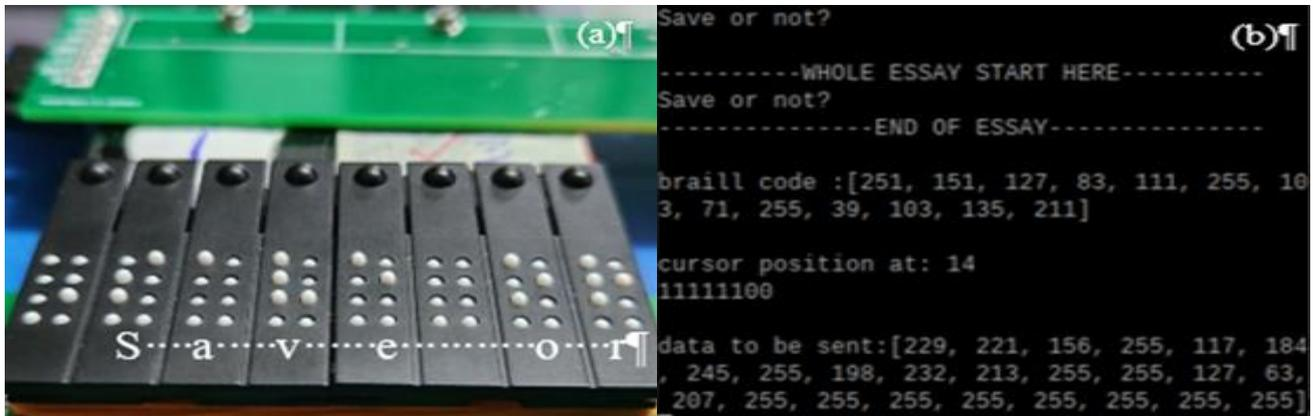
Fig. 5. The text “Save or not?” that shown on (a) the braille cell module and (b) the terminal of Raspberry Pi 4
