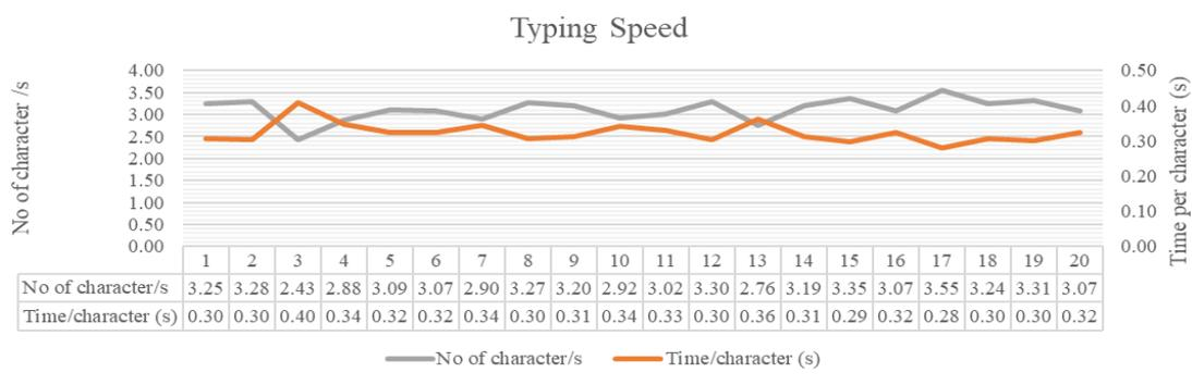
Fig. 6. The typing speed by using the braille notetaker
