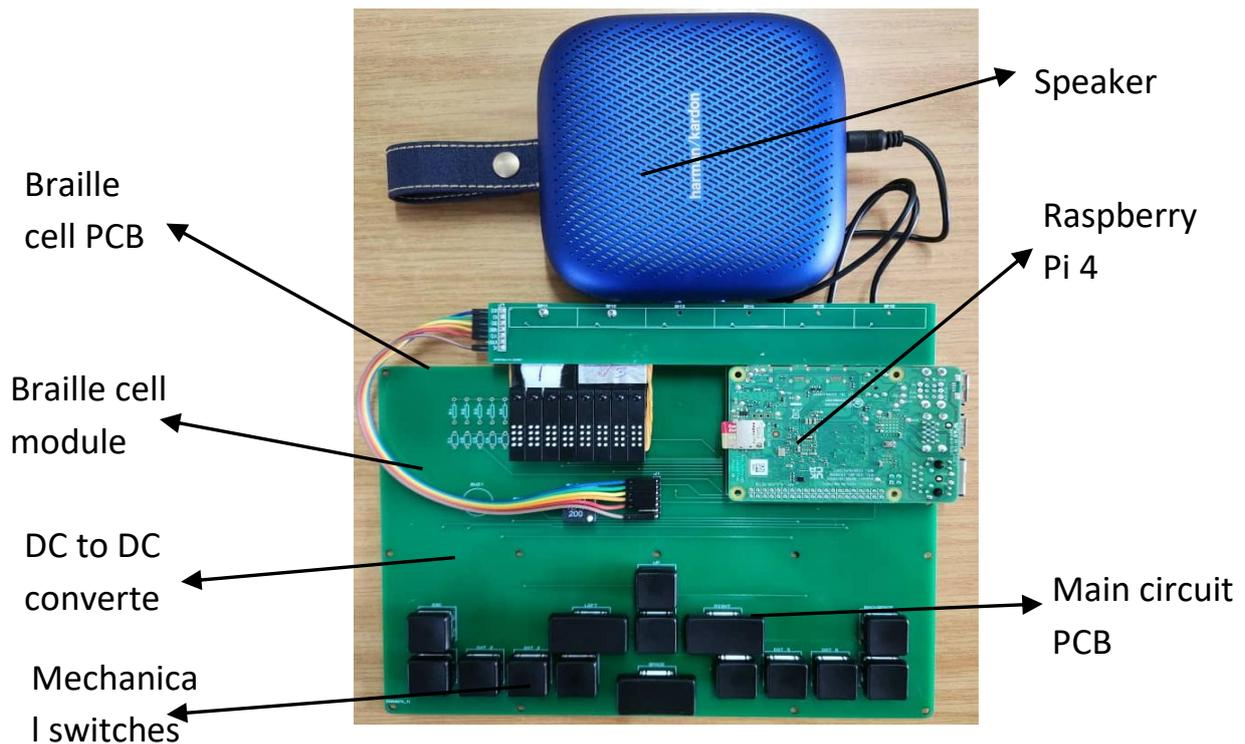
**Fig. 2.** The braille notetaker prototype
