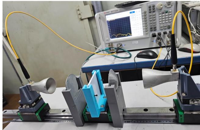
Fig. 12. Measurement setup with lens for 3-D printed horns
