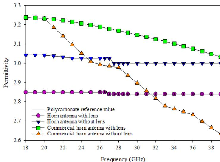
Fig. 23.  $\epsilon_r$  of polycarbonate with and without lens
