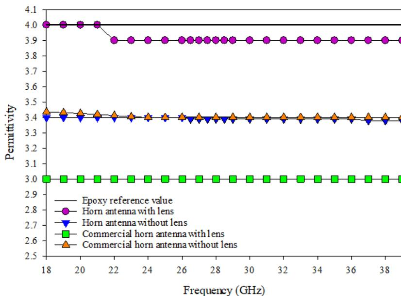
**Fig. 31.**  $\epsilon_r$  of epoxy with and without lens
