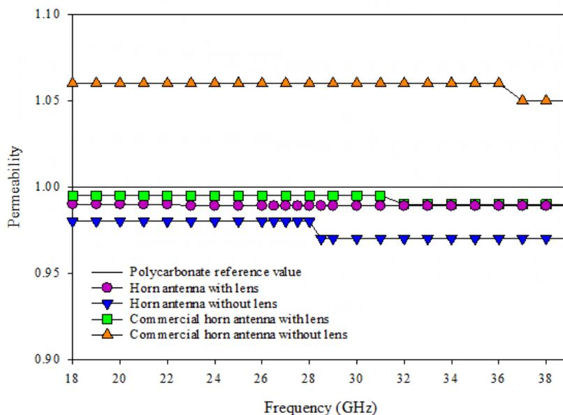
Fig. 24.  $\mu_r$  of polycarbonate with and without lens
