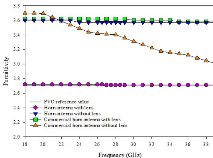
Fig. 25.  $\epsilon_r$  of PVC with and without lens
