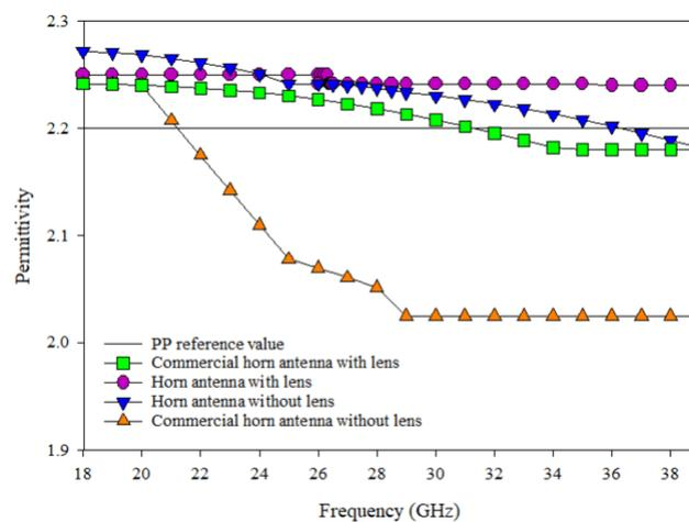
Fig. 19.  $\epsilon_r$  of polypropylene with and without lens
