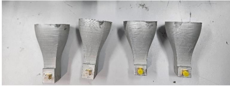
**Fig. 10.** 3-D printed horn antennas
