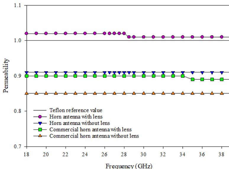
**Fig. 30.**  $\mu_r$  of Teflon with and without lens
