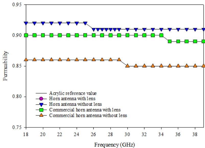
**Fig. 28.**  $\mu_r$  of acrylic with and without lens
