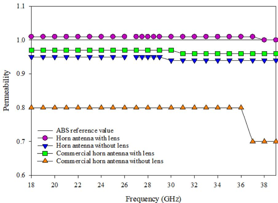
Fig. 22.  $\mu_r$  of ABS with and without lens
