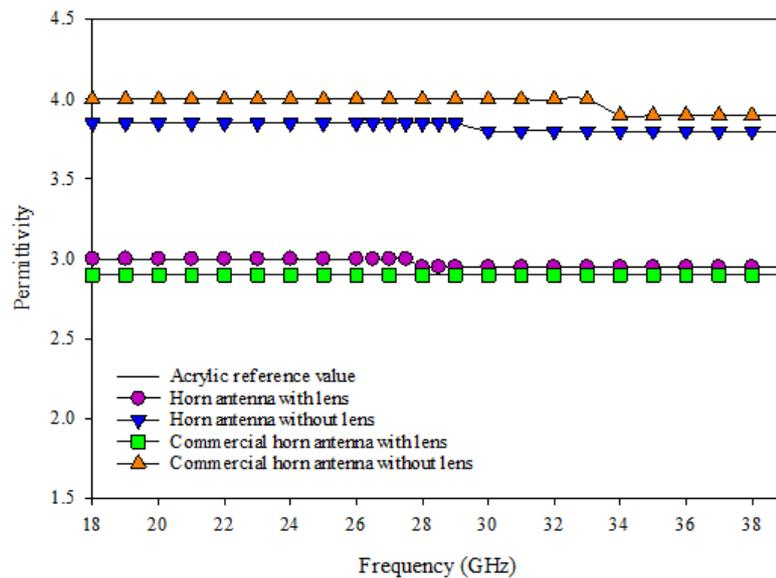
Fig. 27.  $\epsilon_r$  of acrylic with and without lens
