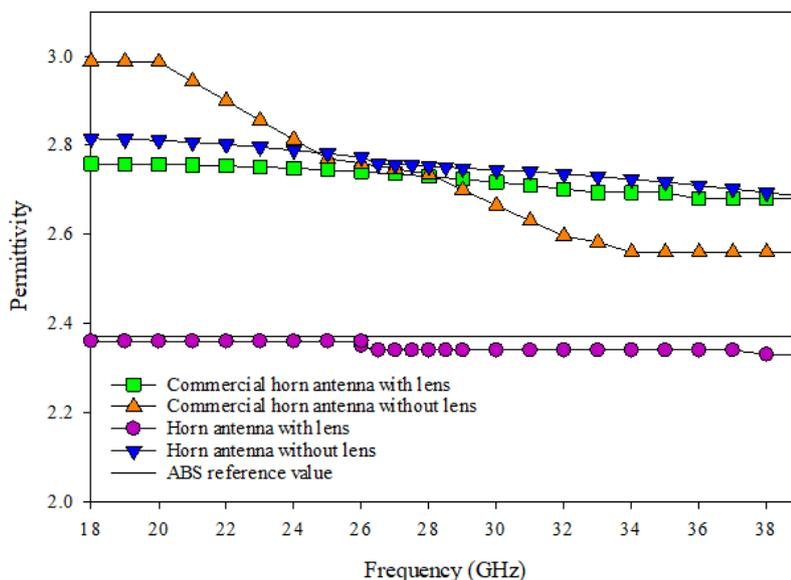
Fig. 21.  $\epsilon_r$  of ABS with and without lens
