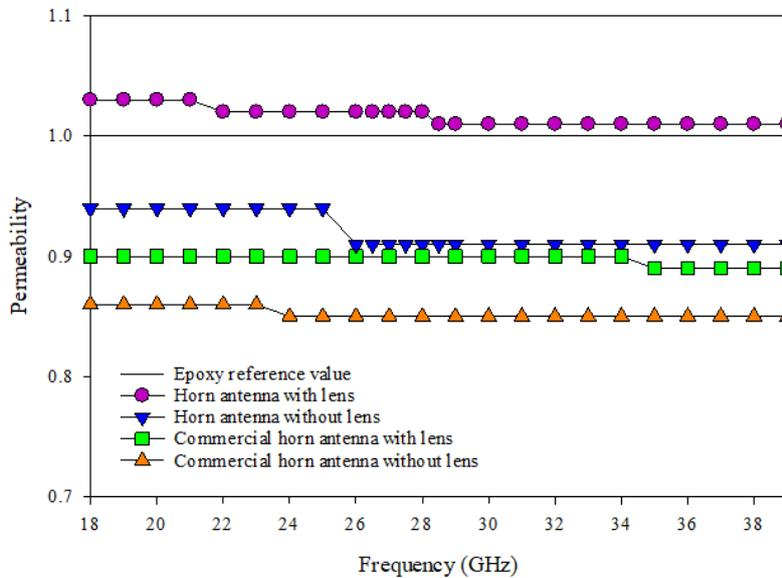
Fig. 32.  $\mu_r$  of epoxy with and without lens
