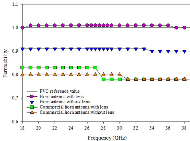
Fig. 26.  $\mu_r$  of PVC with and without lens
