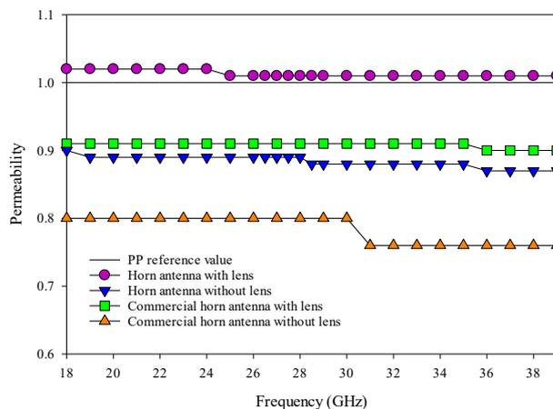
Fig. 20.  $\mu$  of polypropylene with and without lens
