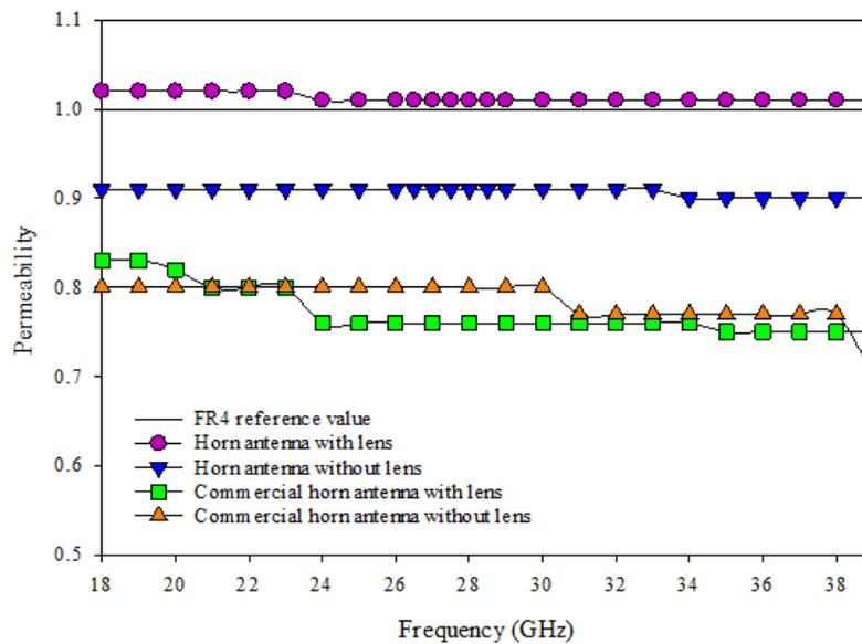
Fig. 18.  $\mu_r$  of FR4 with and without lens
