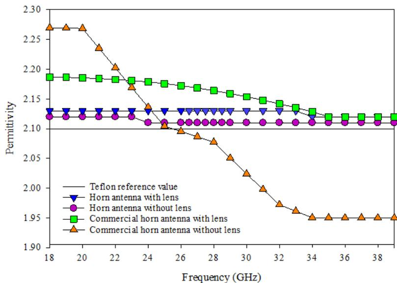
**Fig. 29.**  $\epsilon_r$  of Teflon with and without lens
