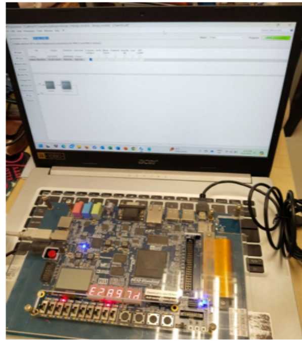
Fig. 10. The connection between the FPGA board and laptop
