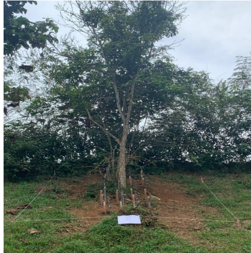
Fig. 2. The installation of tensiometers and gypsum blocks at slope area
