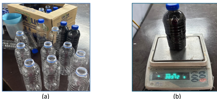
Fig. 1. Material preparation (a) Plastic bottle (b) Weighing plastic bottles filled with 100% rubber chips
