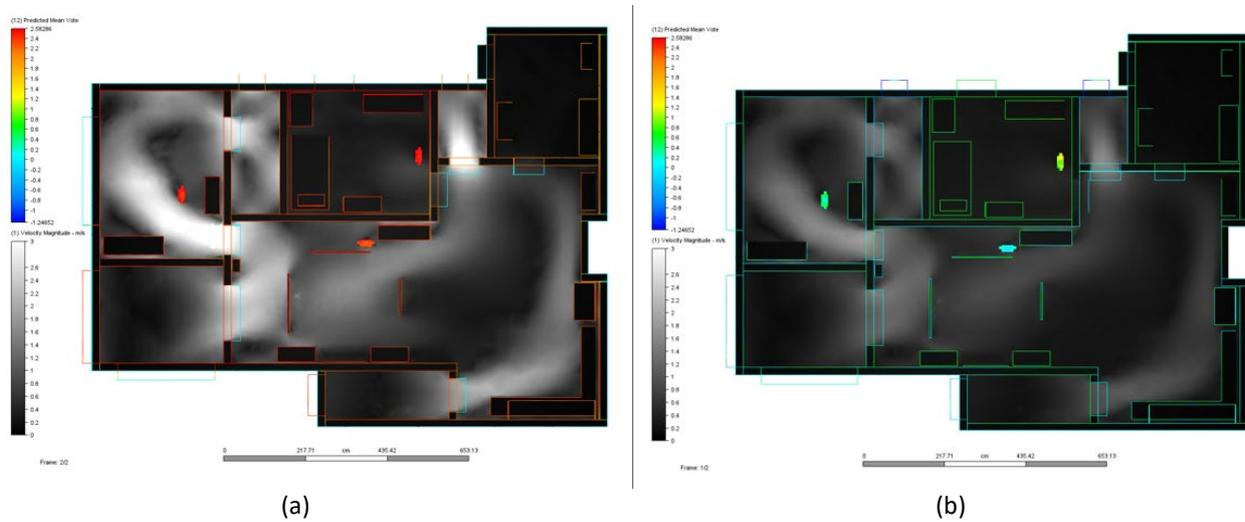
**Fig. 8.** The simulated airflow and the PMV of the occupant for Scenario 3 in (a) daytime and (b) nighttime
