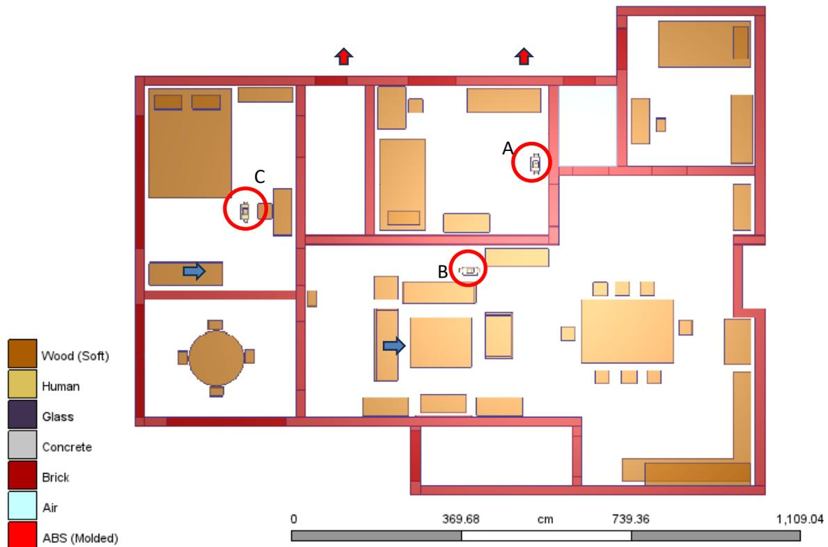
**Fig. 6.** The inlet (blue arrow) and outlet (red arrow) scenario and position of the human models (red circle)
