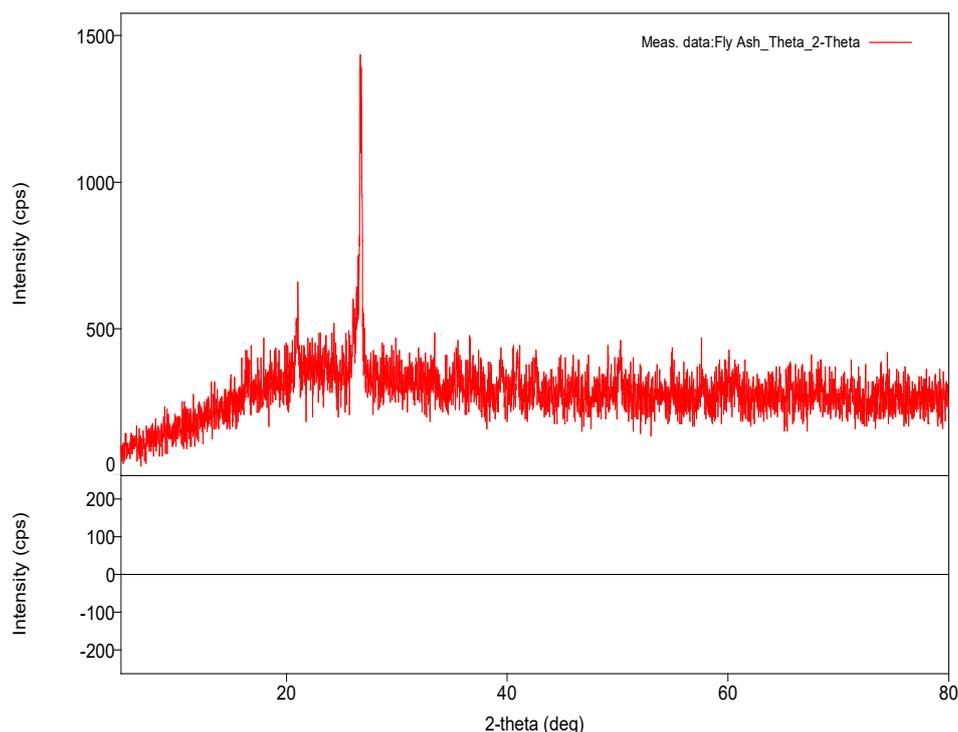
**Fig. 2.** XRD of the fly ash used in this study
