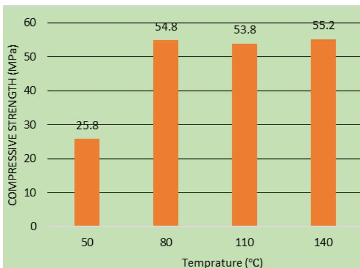
**Fig. 5.** Compressive strength of geopolymer mortar with variations Variation Oven Curing Temperature
