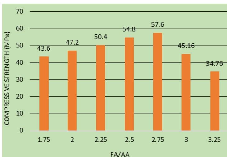
**Fig. 3.** Compressive strength of geopolymer mortar with variations in the ratio of fly ash and alkali activator (FA/AA)
