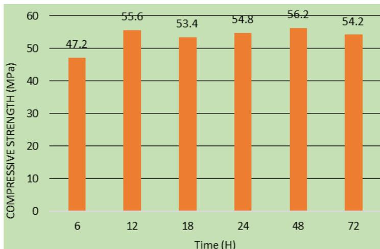
**Fig. 4.** Compressive strength of geopolymer mortar with variations Variation Oven Curing Time
