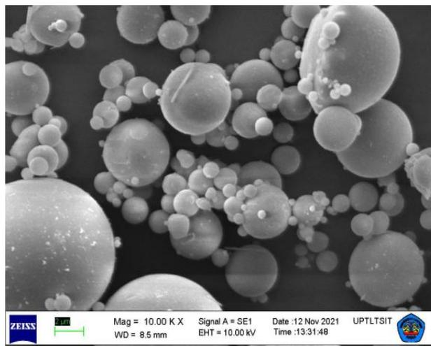
Fig. 1. SEM image of the fly ash used in this study
