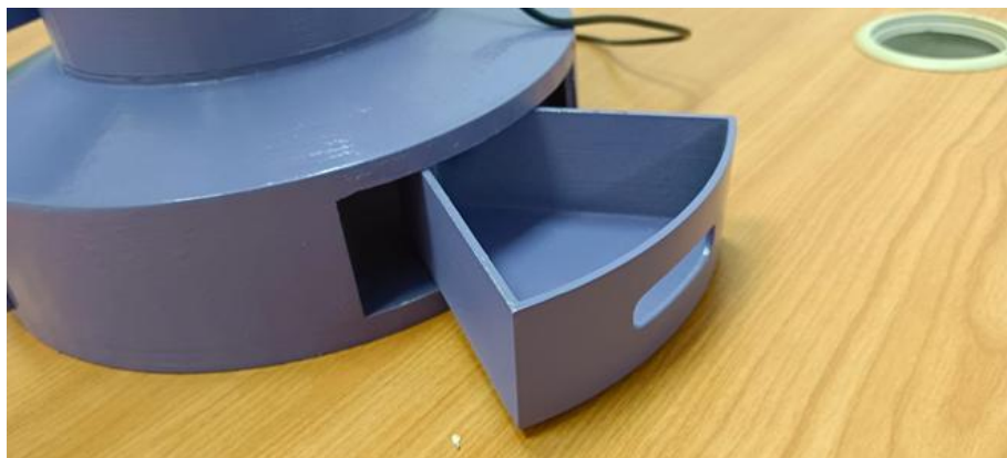
Fig. 15. Drawer sticking issue due to tight tolerances in 3D printed parts
