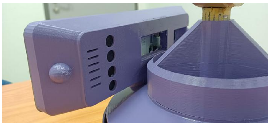
Fig. 14. Measurement error causing battery compartment to not fit, leading to external power wiring
