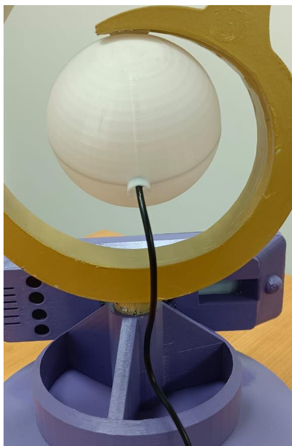
Fig. 12. Exposed wiring after assembling the Ayer Muleh light section
