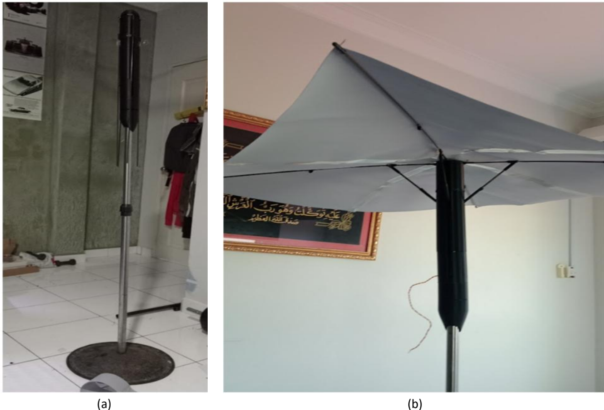
Fig. 6. Figure displays (a) side-view DFED system without the canopy and trusses in closed position (b) the underside the canopy view of the DFED system with exposed wiring
