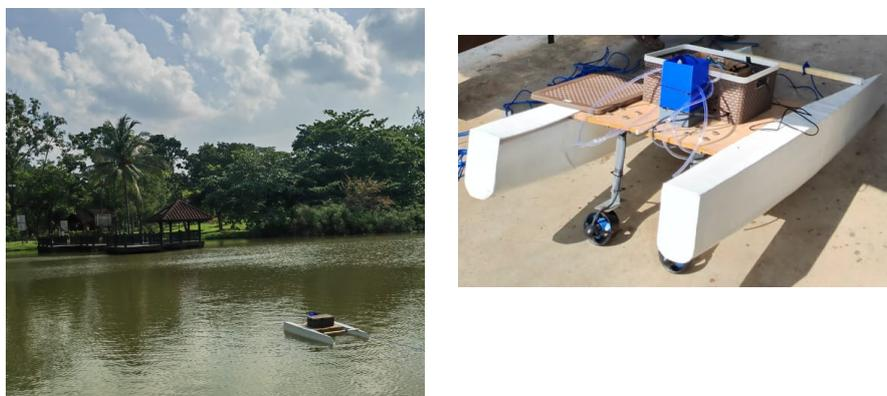
**Fig. 13.** Unmanned Surface Vehicle (USV) prototype used for in situ water quality monitoring
