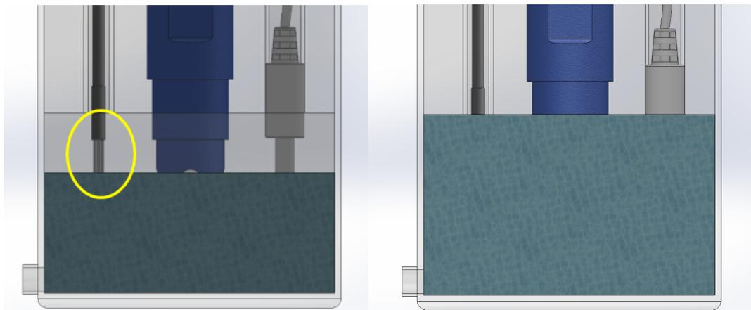
**Fig. 10.** Partially (left) & Fully (right) Submerged Temperature Probe
