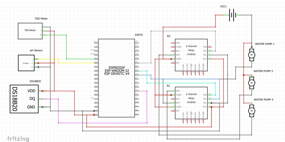
**Fig. 2.** Schematic diagram for in-situ water quality monitoring system
