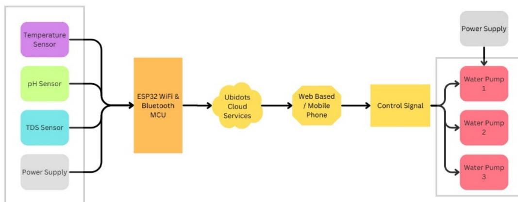
**Fig. 1.** Overview of components for real-time in situ water quality monitoring system
