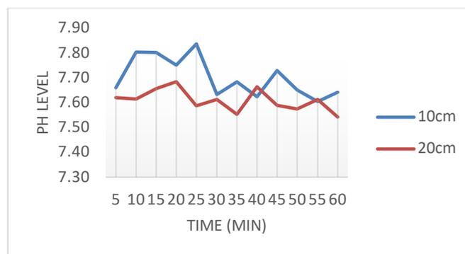
**Fig. 14.** PH level at two different water depth 10cm and 20cm
