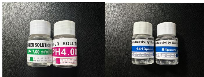
Fig. 5. Buffer Solution for pH and EC for validating the data
