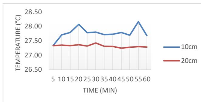
**Fig. 15.** Temperature readings at two different water depth 10cm and 20cm
