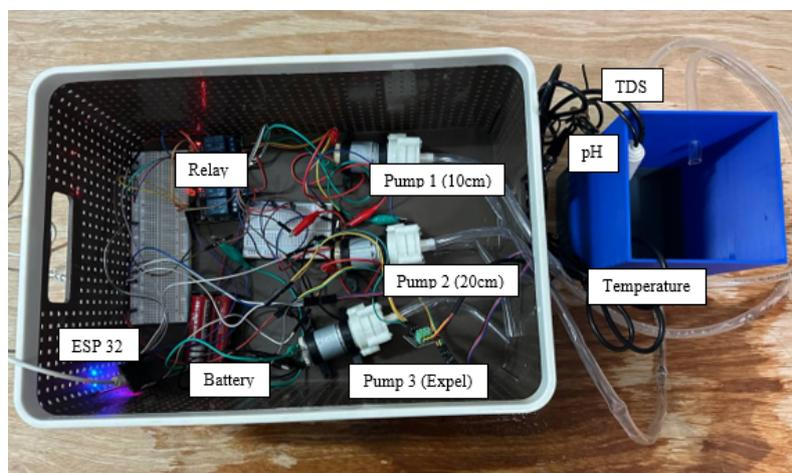
**Fig. 9.** Full setup of prototype for water quality monitoring system
