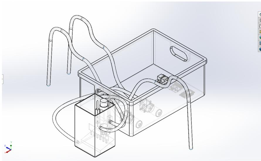
**Fig. 7.** Design of water tank in wireframe mode (SOLIDWORKS)
