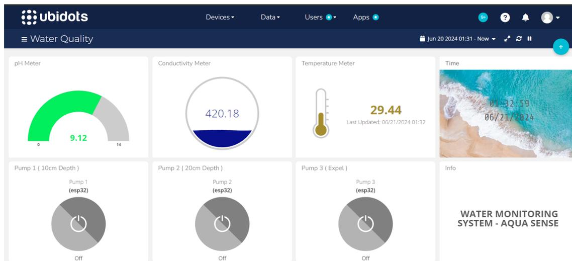
**Fig. 6.** Web-based user interface to monitor water data collection in real-time
