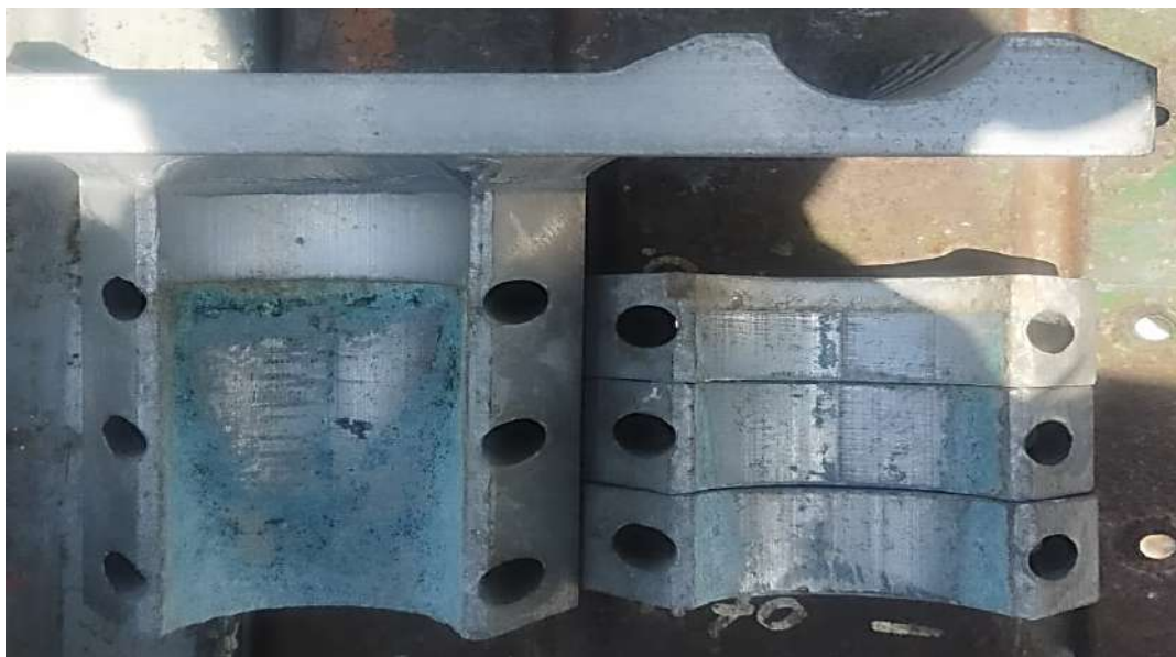
Fig. 4. The clamp section that has corrosion
