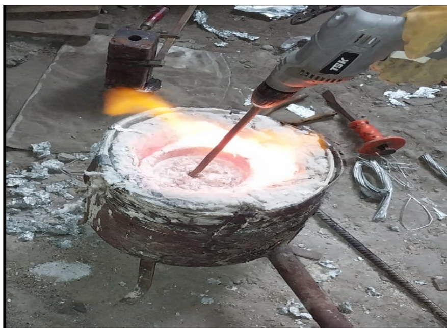
Fig. 1. Casting special alloy of AL 7075
