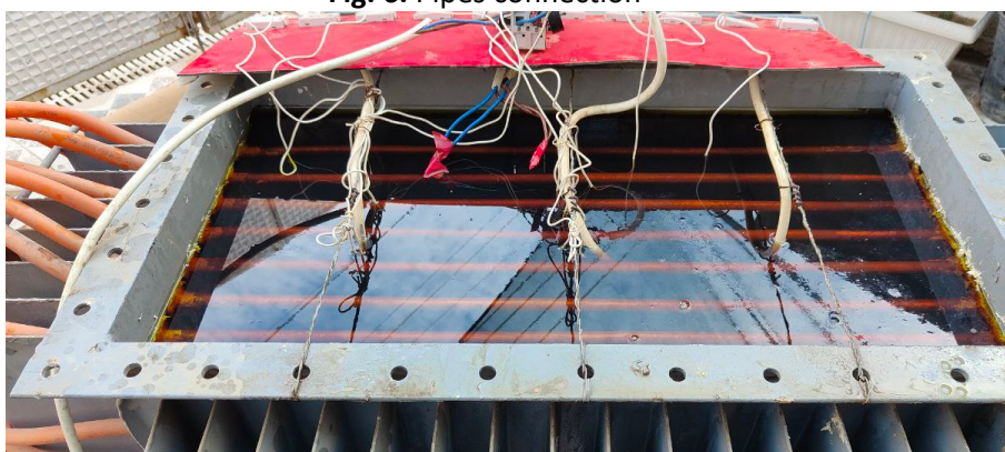
Fig. 7. The transformer tank with pipe immersed in oil
