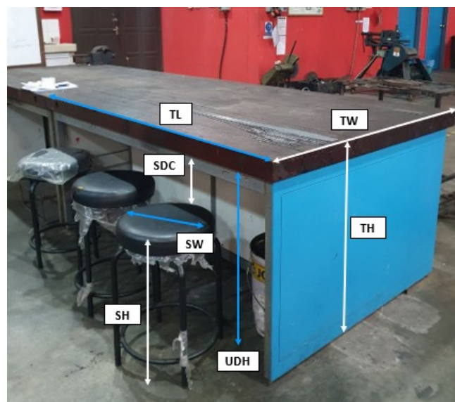
Fig. 3. Dimension labelling of the lab chair and table
