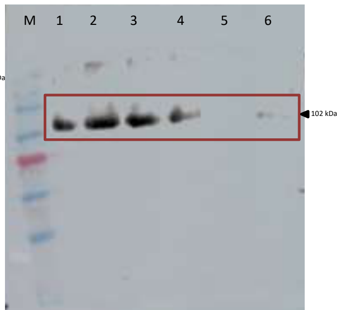
Fig. 18. Western blot result of the insoluble fraction for protein expression in LB media, varying different IPTG concentration and different temperature, where, M: Western marker (PM2700), 1: 0.1 mM IPTG, 16°C, 20 hours; 2: 0.5 mM IPTG, 16°C, 20 hours; 3: 1.0 mM IPTG, 16°C, 20 hours; 4: 0.1 mM IPTG, 16°C, 20 hours; 5: 0.1 mM IPTG, 25°C, 6 hours; 6: 0.1 mM IPTG, 37°C, 4 hours; 7: positive control (Zn Protease protein). The expressed insoluble protein (~102 kDa) bands are highlighted in the red box
