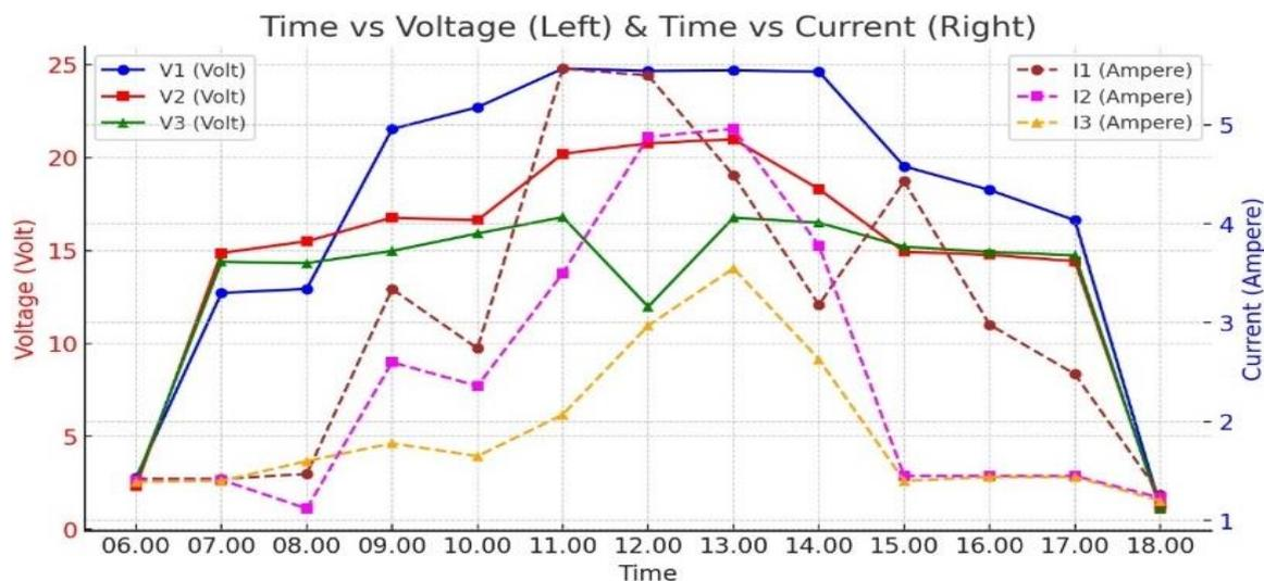
**Fig. 1.** Comparison of current and voltage in monocrystalline, polycrystalline, and thin film
