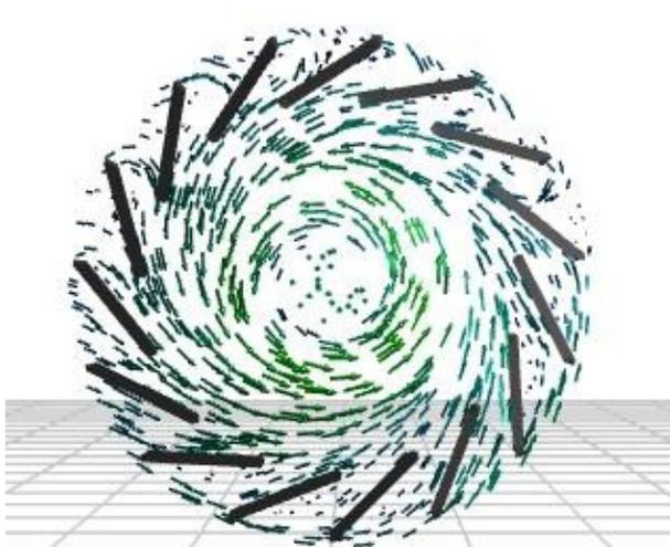
Fig. 8. Velocity vector of coal pulveriser 45° vane
