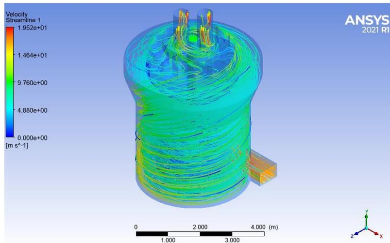
Fig. 7. Velocity streamline of 60° vane angle
