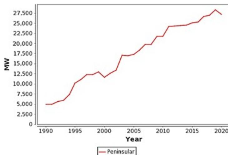
Fig. 1. Total installed energy capacity Peninsular Malaysia
