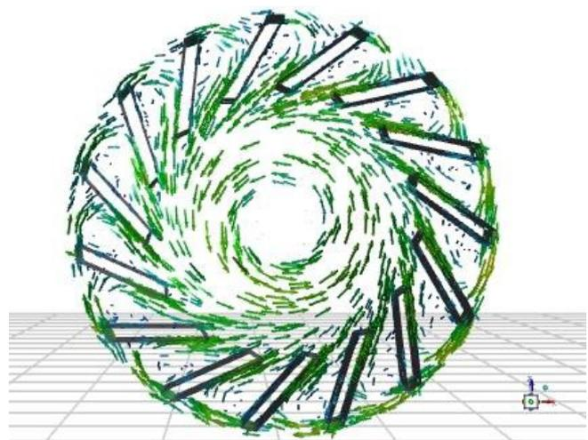
Fig. 9. Velocity vector of coal pulveriser 60° vane
