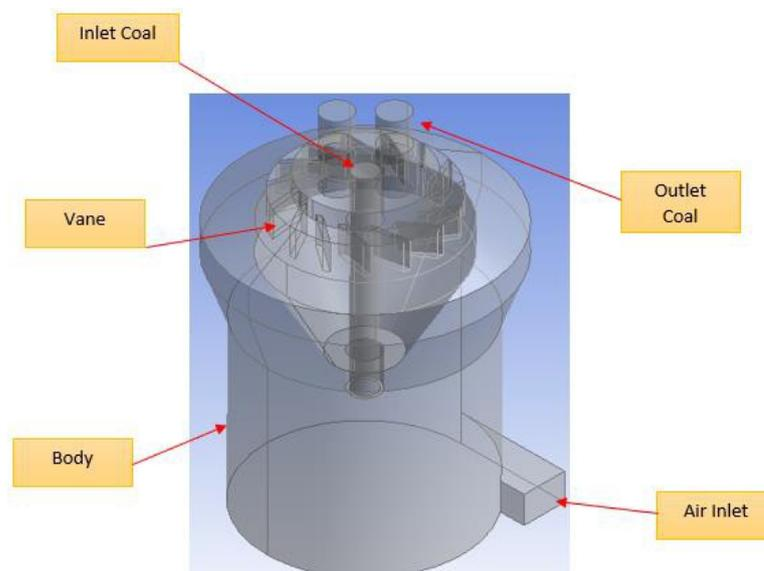
**Fig. 3.** Model of coal pulveriser using SolidWorks software
