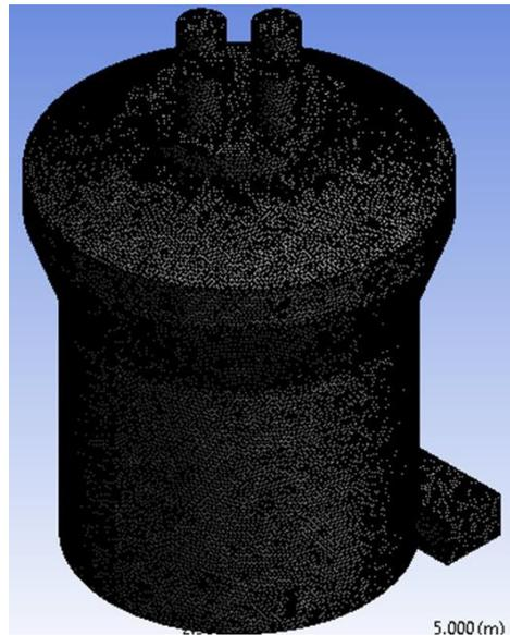
**Fig. 4.** Mesh model for coal pulveriser
