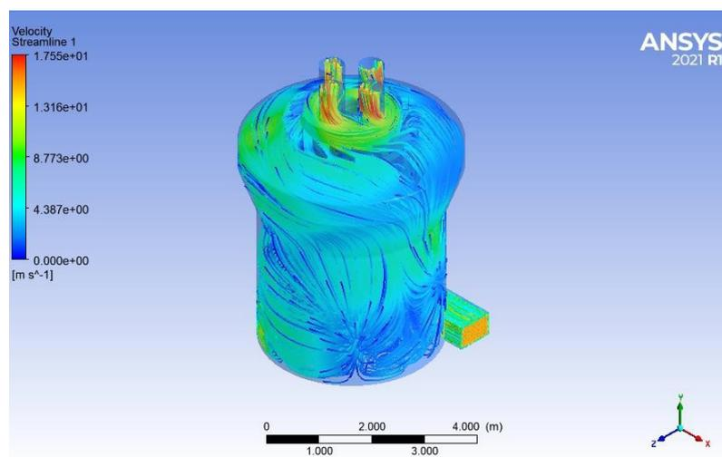
Fig. 6. Velocity streamline of 45° vane angle
