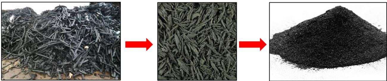
Fig. 1. Material preparation of recycled rubber (RR)
