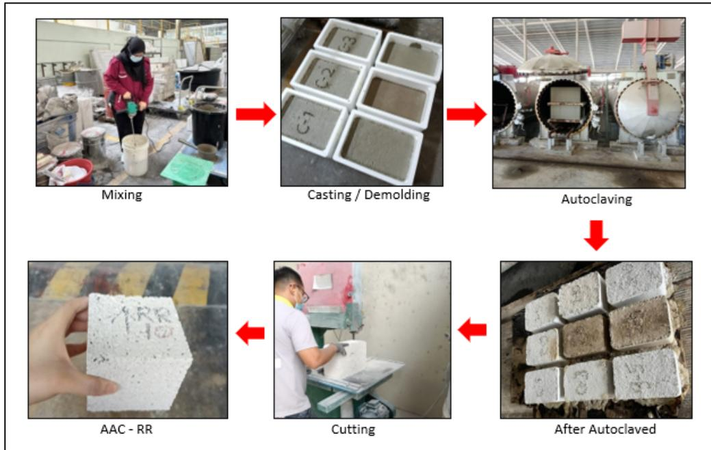
**Fig. 2.** Process of fabrication AAC-RR
