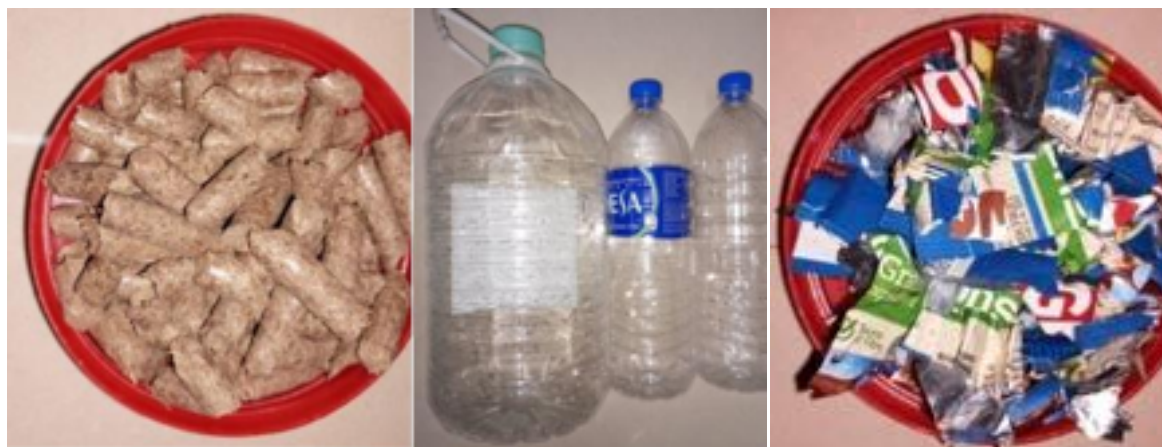
Fig. 1. EFB pellet (left), Polyethylene terephthalate (PET) (middle), Low-density polyethylene (LDPE) (right)
