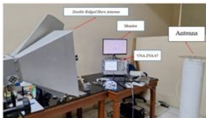
Fig. 17. Measurement setup for antenna
