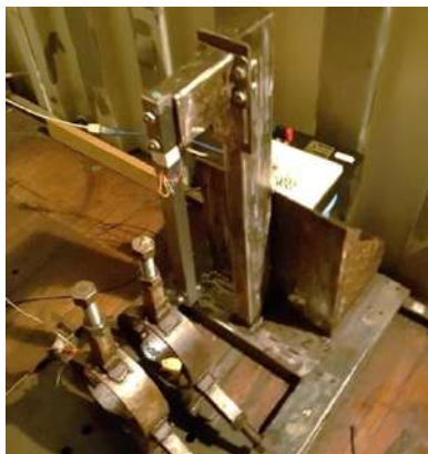
Fig. 1. Solid rocket motors testing bench made at UdeC. Photograph not taken by the author
