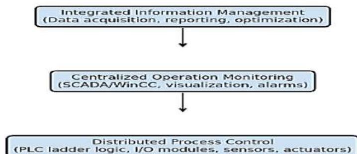
Fig. 5. Layered Architecture of PLC-Driven Electrical Automation System Information, Supervision, and Process Control
