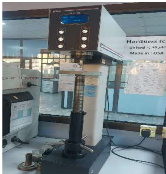
Fig. 4. United HRBW Hardness rig machine
