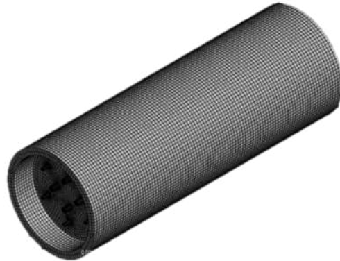
Fig. 2. Discretised computational domain illustrating the uniform structural mesh in both axial and radial directions. A global element size of 30 mm was implemented to ensure numerical accuracy while maintaining computational feasibility for the coupled reacting-flow simulations.
