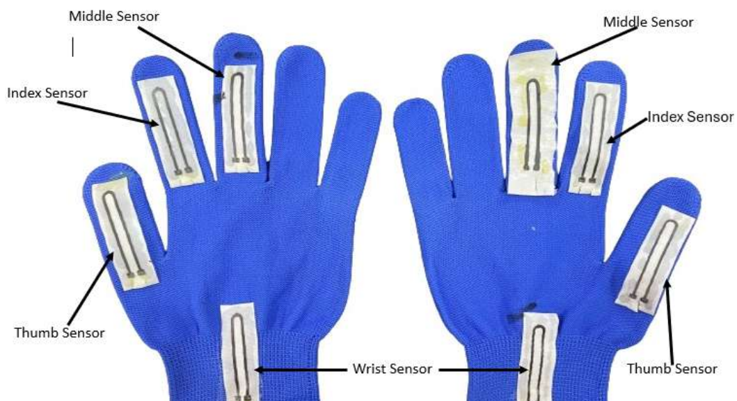
Fig. 1. Stretchable strain sensor- based glove with the developed sensors
