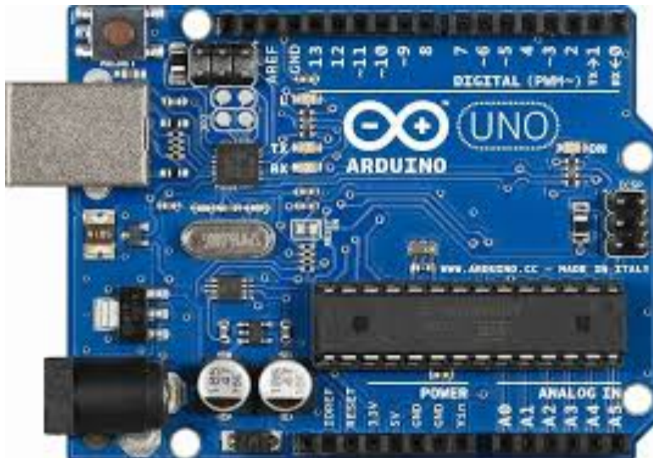
Fig. 4. Arduino Uno R3 based on the Atmega328P
