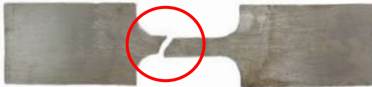
Fig. 8. Deformed Specimen after Uniaxial Tensile Test
