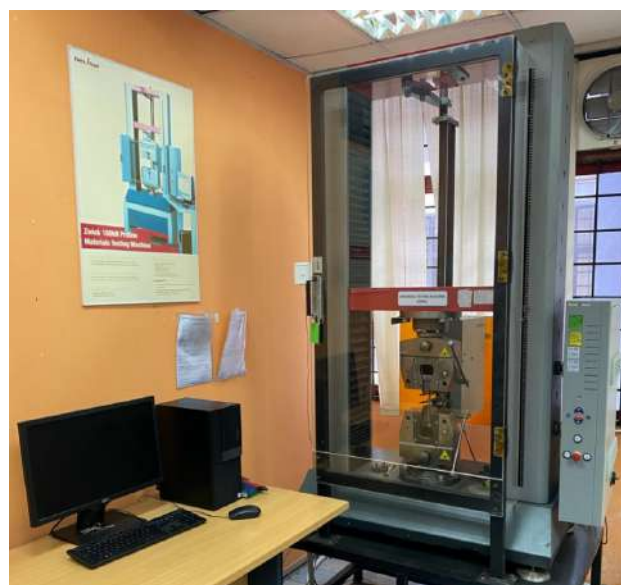
Fig. 3. Zwick Roell Z030 Universal Tensile Testing Machine 10KN
