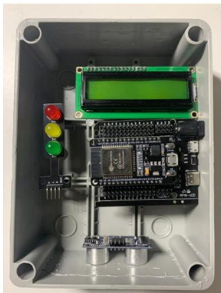
Fig. 1. Physical assembly of the FRMS hardware node including the ESP32 microcontroller, HC-SR04 ultrasonic sensor, 16x2 LCD screen, and traffic-light LED alert module
