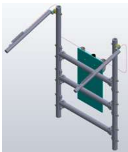
Fig. 2. The CAD model (solid) of the proposed exoskeleton. All electronic components are placed at the back plate (in green)
