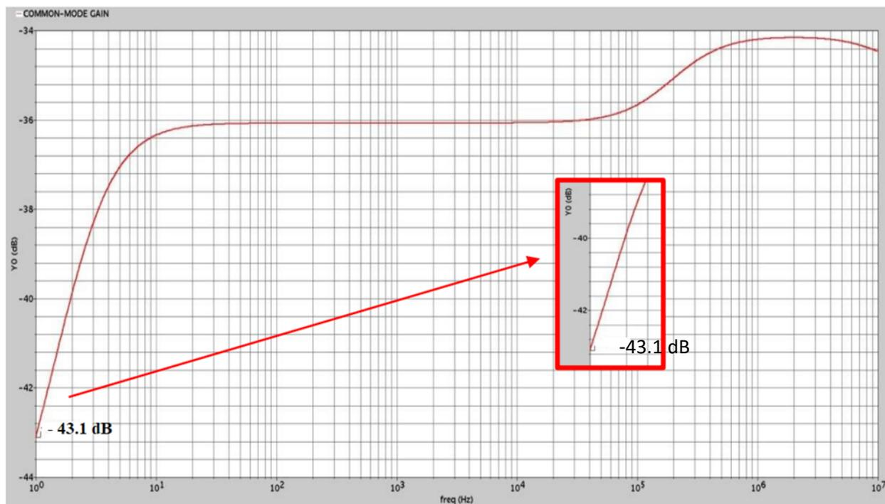
**Fig. 8.** Common mode gain of the instrumentation amplifier (pre-layout)
