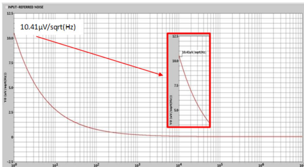
Fig. 7. Input referred noise of instrumentation amplifier (pre-layout)
