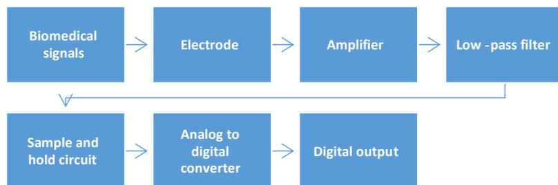
**Fig. 2.** Biomedical electronics detecting system blocks
