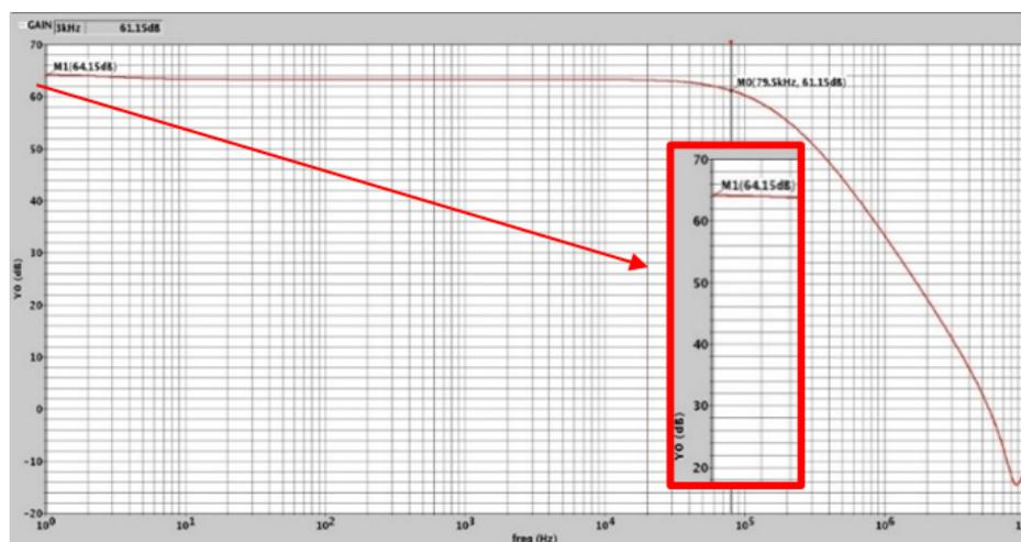
**Fig. 5.** Differential gain of the proposed instrumentation amplifier (pre-layout)
