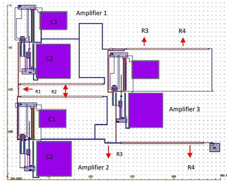
**Fig. 9.** Layout of proposed instrumentation amplifier
