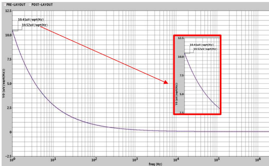
**Fig. 11.** Input referred to noise of instrumentation amplifier (pre-layout & post-layout)
