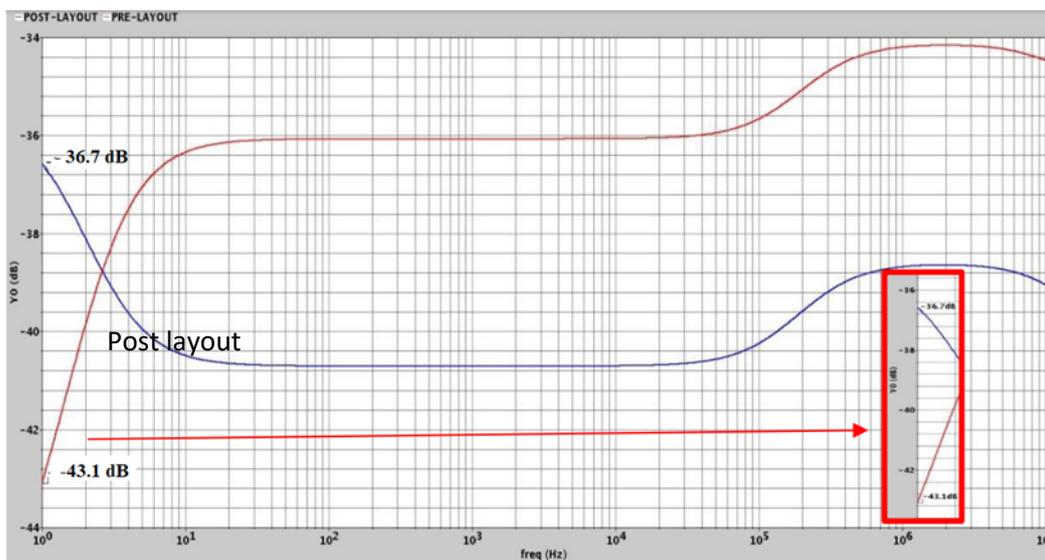
**Fig. 12.** Common mode gain of the instrumentation amplifier (pre-layout & post-layout)
