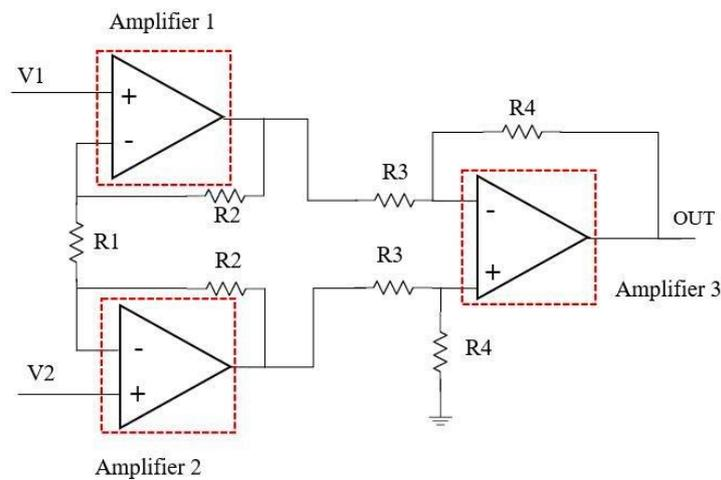
**Fig. 1.** Schematic diagram of instrumentation amplifier
