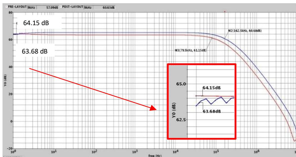
**Fig. 10.** Differential gain of the instrumentation amplifier (pre-layout & post-layout)
