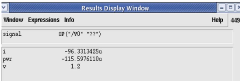
Fig. 6. Power dissipation of instrumentation amplifier (pre-layout)
