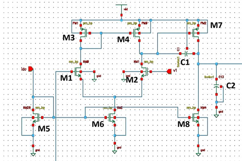
Fig. 3. Schematic of two-stage CMOS op-amp
