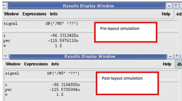
**Fig. 13.** Power dissipation of instrumentation amplifier (pre-layout & post-layout)
